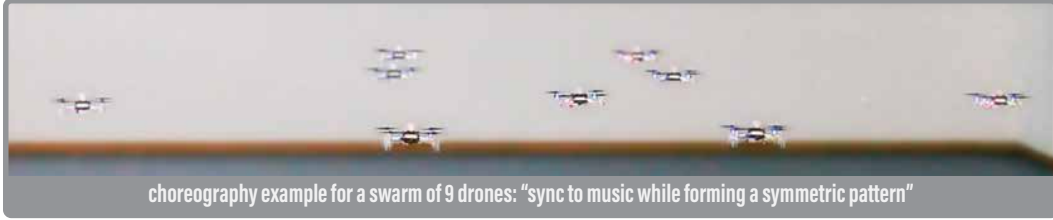
Figure 1: Choreography of a 9-drone swarm by Swarm-GPT. Formations shown in the picture are synchronized to the music beat times. Users can interact with Swarm-GPT to generate different trajectories. Full experimental performance available from the video: http://tiny.cc/Swarm-GPT
