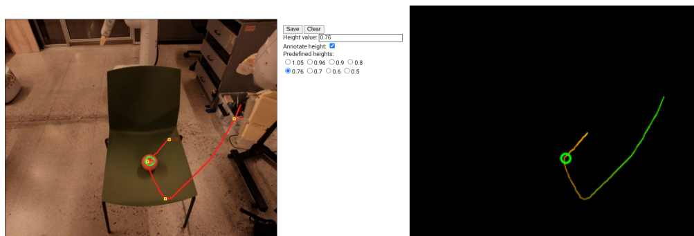
Figure 6: Left: The GUI for users to draw trajectory sketches given the robot’s current camera image. The 2D trajectory is directly drawn by manual input, which can then be annotated with interaction markers or waypoints corresponding to user-specified heights. Right: The resulting height-aware trajectory sketch generated according to the output of the UI.
