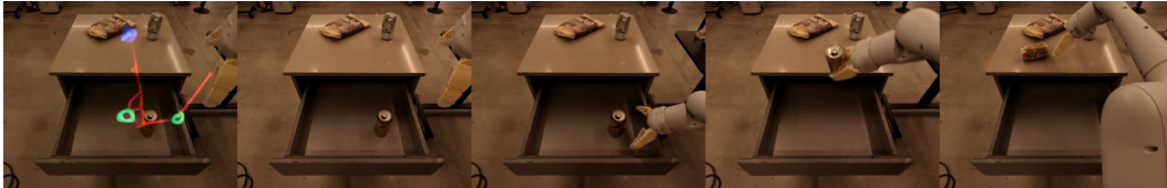
Figure 5: Example trajectory from image generation models. From left to right, the first image shows the overlaid trajectory sketch, and the next 4 images show the rollout conditioned on it. The language instruction is: pick orange can from top drawer and place on counter.
