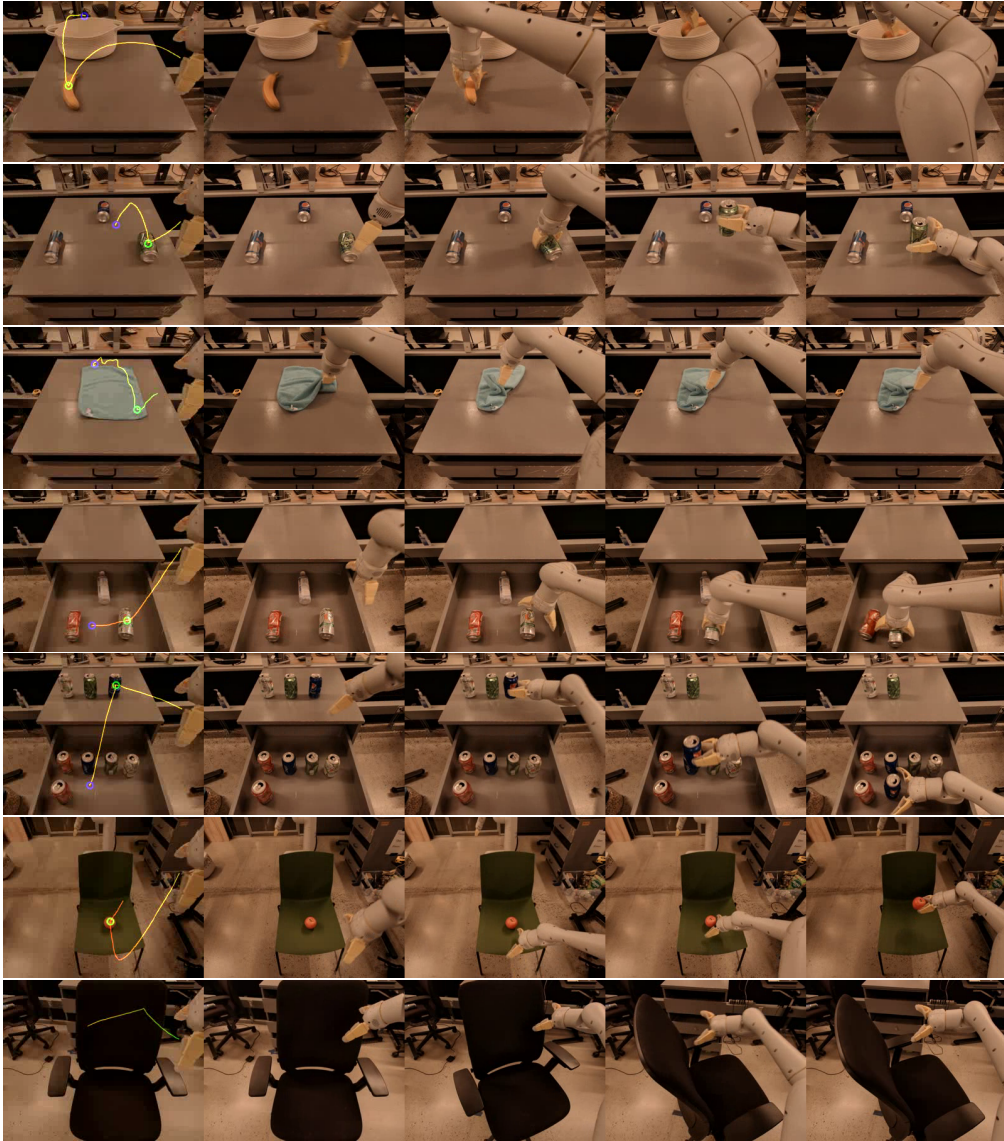
Figure 7: Example rollouts of 7 unseen skills. The trajectory sketch overlaid on the initial image is visualized. From top to bottom: Place Fruit, Upright and Move, Fold Towel, Move within Drawer, Restock Drawer, Pick from Chair, Swivel Chair.
