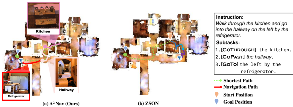
Figure 12: Visualization of the navigation path. Our method successfully goes through the kitchen and finds the refrigerator, while the baseline fails to do it.
