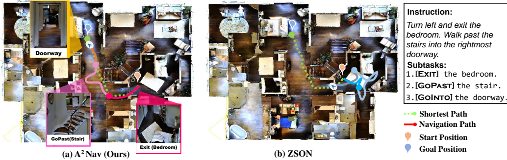
Figure 11: Visualization of the navigation path. Our method successfully exits the bedroom and goes past the stair, while the baseline is stuck in the bedroom.
