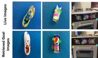
Figure 3: In each column, given a live image (top) DINOBot retrieves from the buffer the most similar image in the buffer (bottom), and finds correspondences between the two.
