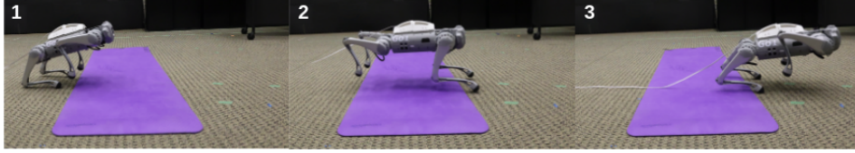
Figure 3: Using the bounding gait, the robot can jump over a 60cm-wide yoga mat without making foot contact.
