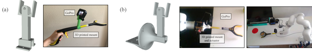
Figure 4: In part (a), we show the setup for collecting human demonstrations. This includes a 3D printed mount, a camera, and the reacher-grabber stick. Part (b) displays the corresponding setup on the robot.
