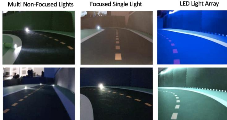
Figure 3: The camera capture from robocar’s perspective for testing varying sim2real environments.
