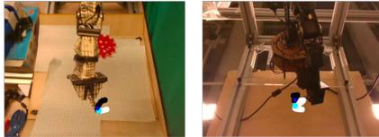
Figure 8: [Best seen in pdf] Robot-to-robot imitation with MAVRIC. In both video frames, cyan represents the next target, white points are future target points, and black points are previously reached target points. **(left)** A video frame of a source robot draws the letter C — in this case, we used MAVRIC to perform this task with visual servoing for trajectory-following. **(right)** A video frame of the target robot imitating the motions of the source robot. Full video in Supp.
